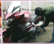
ACF-50 is used on motorcycles just like aircraft. Application under panels and to hidden areas is as important as treating the exposed parts. ACF-50's chemistry protects the engine case/cooling fins, gear case, radiators and forks,...all corrosion prone areas.
